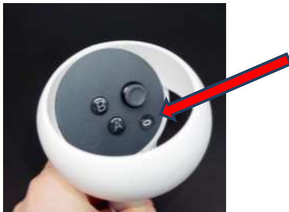
Figure 40 - Analog stick and three additional buttons “A”, “B”, “O” on the manipulator
